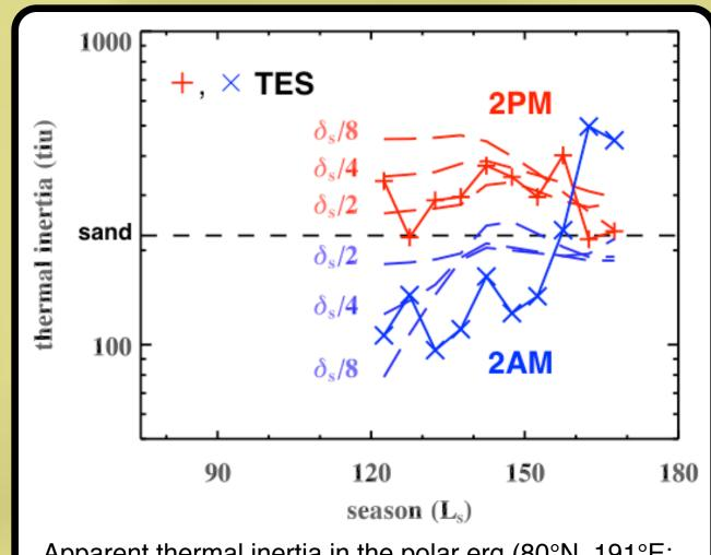
Apparent thermal inertia in the polar erg (80°N, 191°E + in maps) from TES and layered models of sand over ground ice, with best-fit of ~20 cm of sand.
