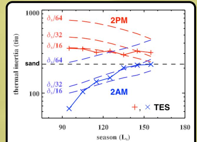
2AM and 2PM seasonal apparent thermal inertia at Phoenix from TES and layered models of sand (223 tiu) overlying ground ice (2506 tiu). Model surface-layer thickness is given in fractional seasonal skin depth, δs (70 cm for sand). Best-fit model has ~4 cm of sand. Seasonal range is limited by transient CO<sub>2</sub> frost.
